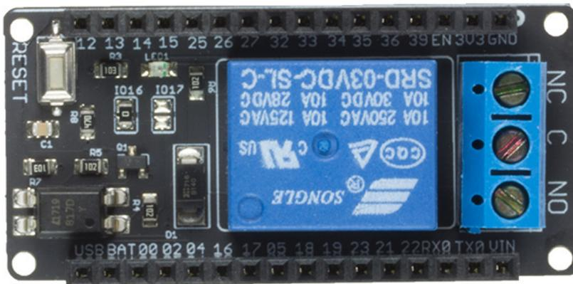
This is an opto-isolated relay board driven by a single digital pin. It is a 110V, 10A maximum AC relay board in the IoT-Bus form factor.
